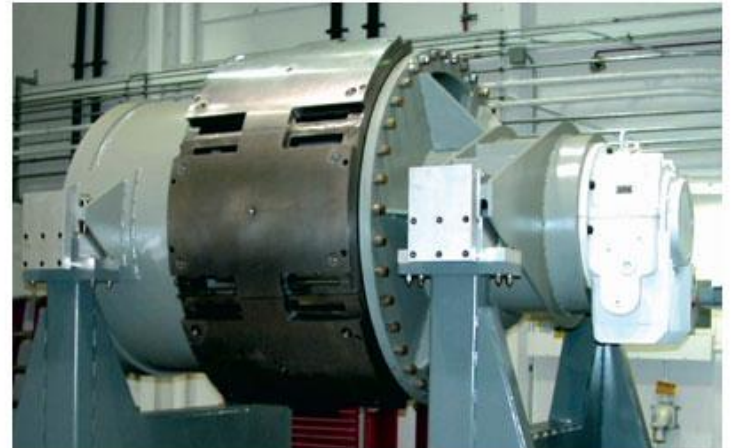
One-quarter scale 5,000 hp motor under construction
